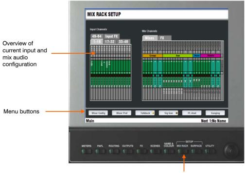
To access the MixRack audio configuration press the MIXRACK SETUP key below the TouchScreen.
